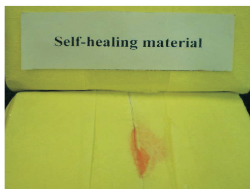
Figure 4 self-healing demonstration sample.
