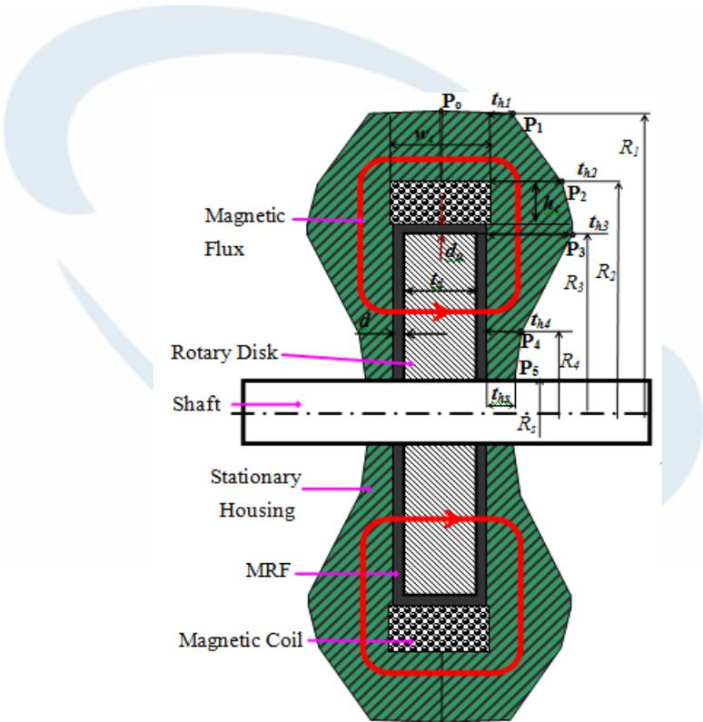
Figure 2. Configuration of a disc-type MRB with 5-segment polygonal envelop
