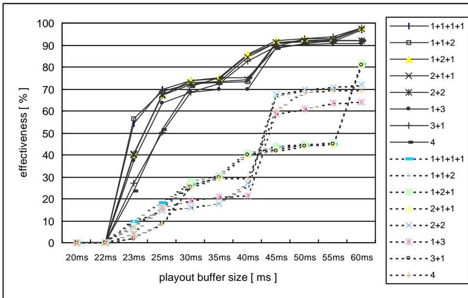
Fig 10 The effectiveness error recovery in L4, the dotted lines represent unicast-based, and the black thin lines represent subcast-based.
