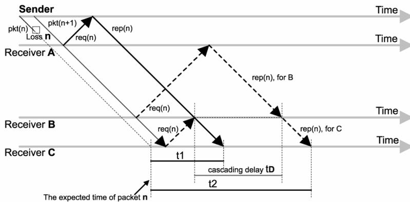
Fig 4 The timing diagram about the error recovery behavior both unicast (the dotted lines) and subcast (the black thick lines).
