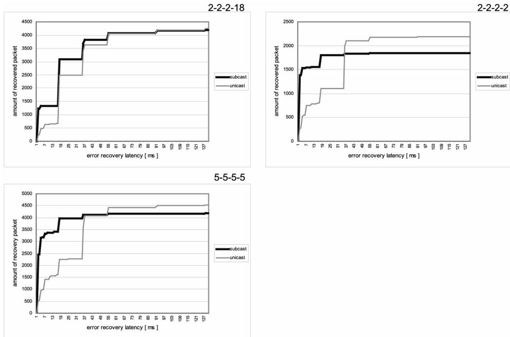
Fig 8 The CDFs of error recovery latency.
