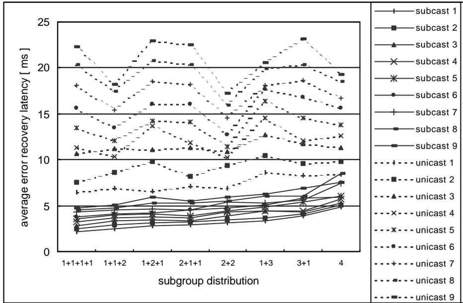
Fig 7 The average error recovery with increasing delay at the link in L4.
