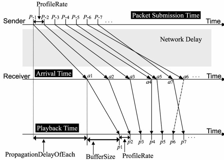
Fig 9 The transmission model for evaluating the effectiveness.
