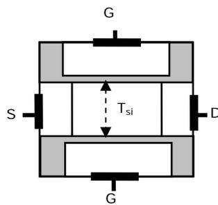
Fig. 11. Double-gate device structure with independent gates.
