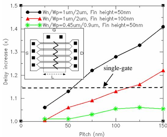
Fig. 7. Effect of distributed gate resistance on inverter delay for different device widths, fin heights, and pitch sizes. Insert shows inverter layout in FinFET implementation.
