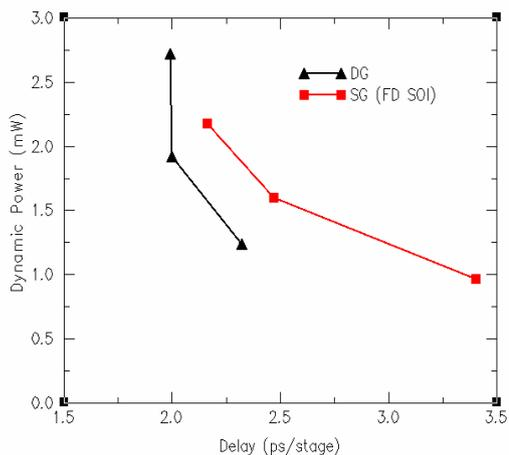
Fig. 6. Power-delay for inverter ring oscillator for 45nm technology with  $V_{dd} = 0.4, 0.6, \text{ and } 0.8 \text{ V}$ .
