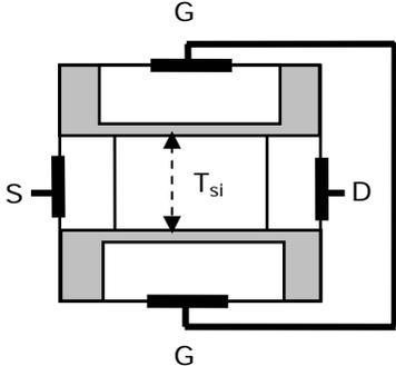
Fig. 1. Double-gate device structure with tied gates.
