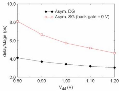
Fig. 10. Model-predicted inverter delay vs.  $V_{dd}$ .
