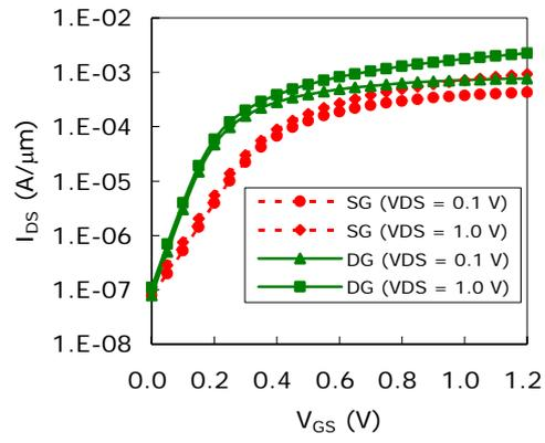
Fig. 12. MEDICI-simulated nFET  $I_{DS} - V_{GS}$  characteristics at  $V_{DS} = 0.05$  and 1 V for double-gate (DG) (tied gates) and single-gate (SG) (back-gate biased at 0 V) modes.
