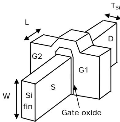
Fig. 3. FinFET device structure.
