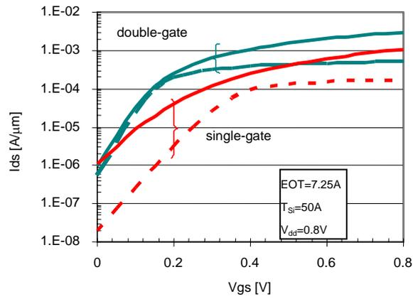
Fig. 4. I-V characteristics of FinFET (double-gate) and single-gate FDSOI device. with 18 nm gate length and 0.8 V power supply.
