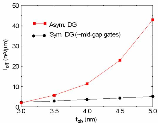
Fig. 8. Model-predicted  $I_{off}$  vs. back-oxide thickness variation.
