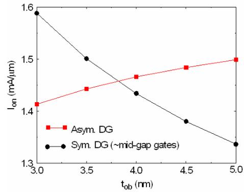
Fig. 9. Model-predicted  $I_{on}$  vs. back-oxide thickness variation.
