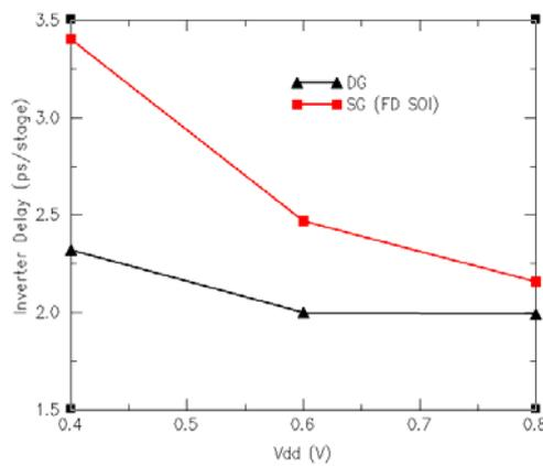
Fig. 5. Inverter delay for FinFET (DG) and FDSOI devices for different power supplies. Device width has been adjusted for  $I_{on} = 3$  mA (Distributed gate resistance is not included).
