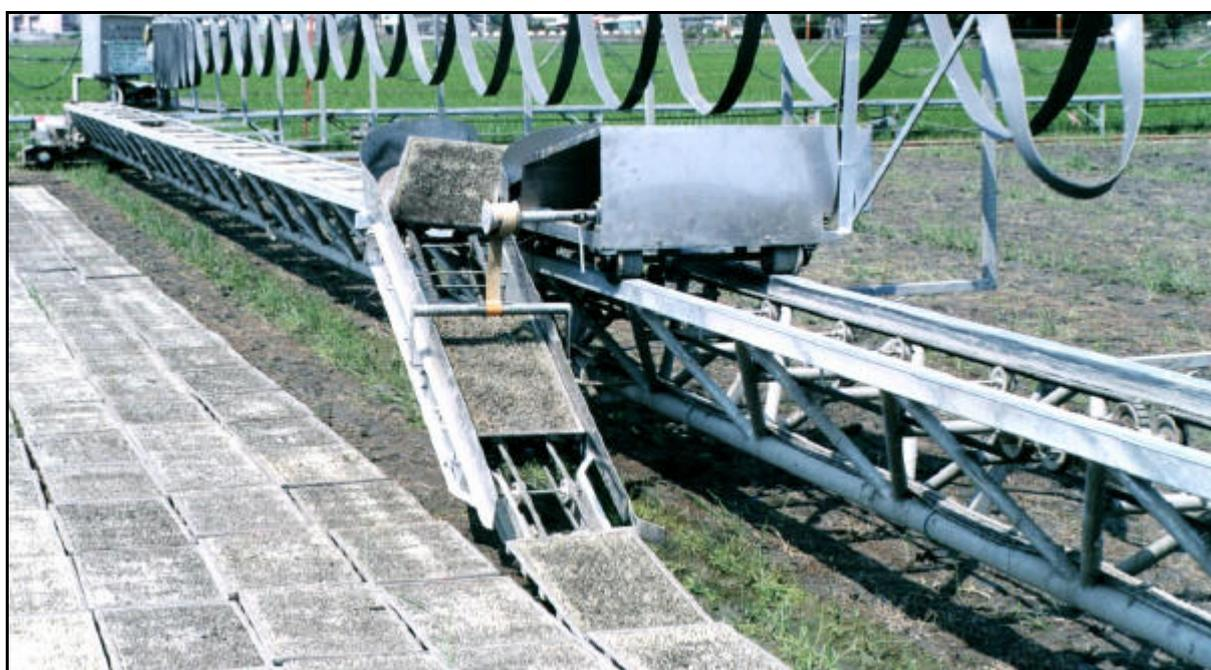
Figure 1 Photograph of the subject gantry in field operation.
