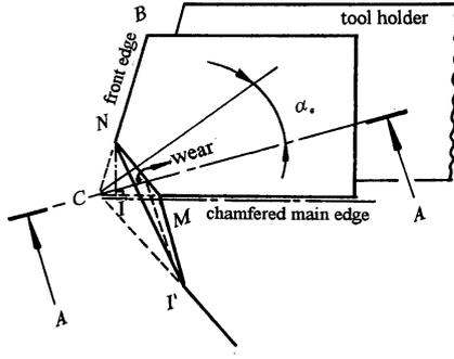
Figure 3. Tool tip wears with chamfered main cutting edge tool.
