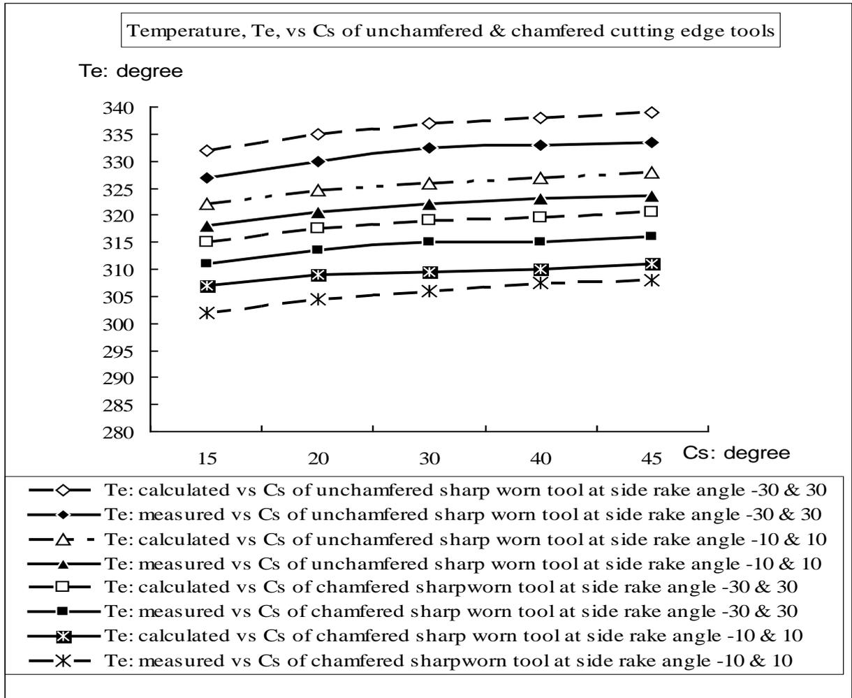
Figure 7. Shows the cutting temperatures vs  $C_s$  for different values  $\alpha_{s1}$  and  $\alpha_{s2}$  with chamfered and unchamfered sharp tool at  $d=3.0$  mm,  $f=.33$  mm/rev,  $V=252$ m/min respectively.
