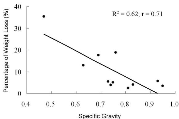
Fig. 2 Correlation of specific gravities and percentages of weight loss of hardwood species tested
