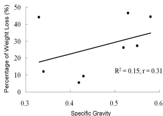
Fig. 3 Correlation of specific gravities and percentages of weight loss of softwood species tested
