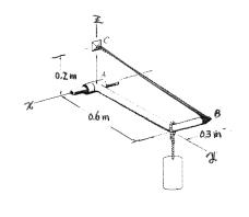
2. Member AB as shown in Fig. d Problem 1, is supported by a cable BC and a A by a square rod, which fits loosely through the square hole at the end joint of the member as shown. Determine the components of reaction a A and the tension in the cable needed to hold the 800N cylinder in equilibrium. (30%)
